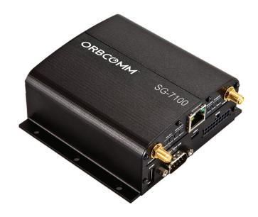
The SG-7100 cellular communications gateway is a powerful cellular platform with optional Wi-Fi and satellite, providing broadband connectivity for easy integration into fleet management and industrial fixed asset monitoring applications.
